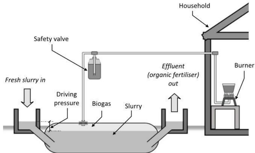
Figure 1: Sketch to show the basic workings of a simplified domestic biodigester
