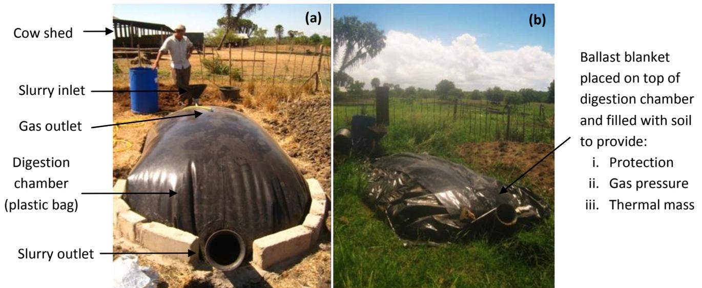
Figure 4: Photos of a prototype flexible bag digester (a) without the ballast bag and (b) and with it in place
