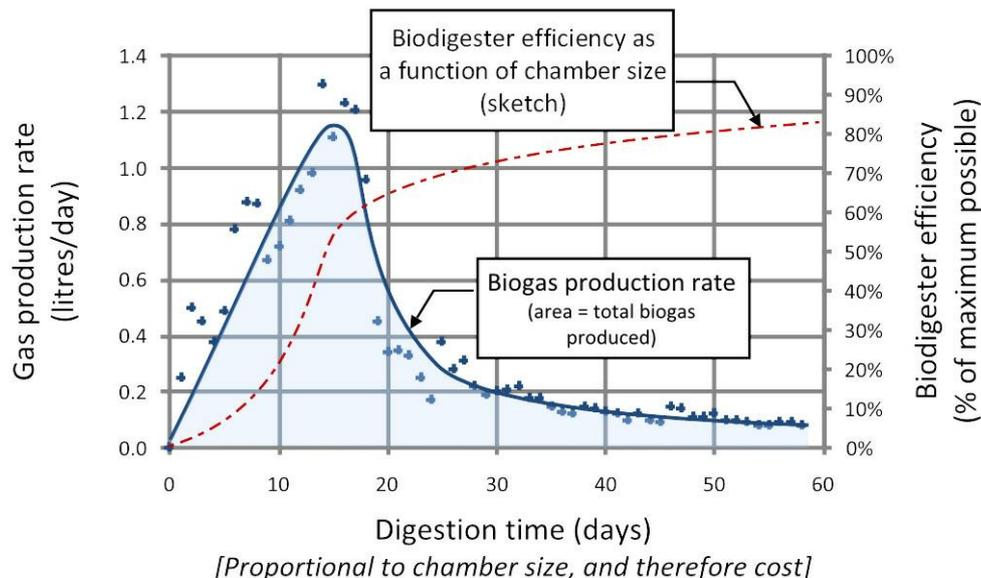
Figure 5: Biogas production for 1 litre of slurry as it moves through a biodigester, along with the cumulative biodigester efficiency at each point. Data points taken from (8).
