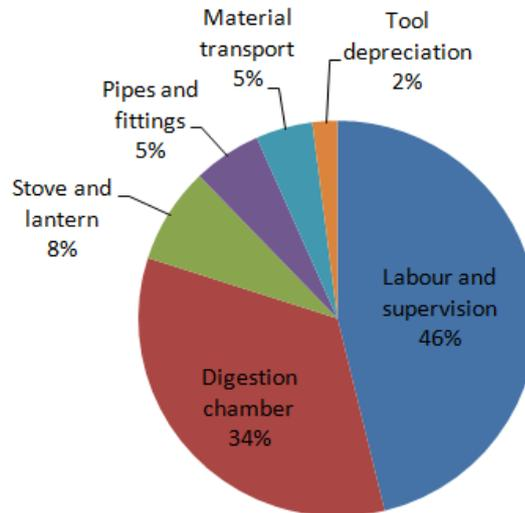
Figure 3: Relative cost of all aspects of fixed dome biodigester, created from a parts list in (4)
